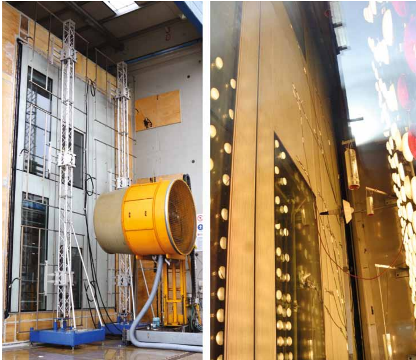
Figure 3: TEC performance test: dynamic water penetration test (left) and thermal cycle test (right)
